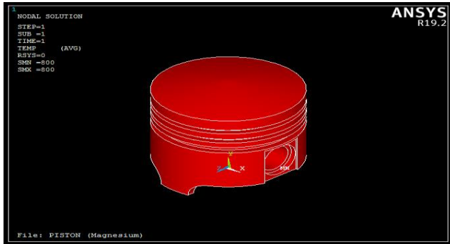
Fig. 7.6: Nodal Temperature of Piston – Magnesium Alloy
