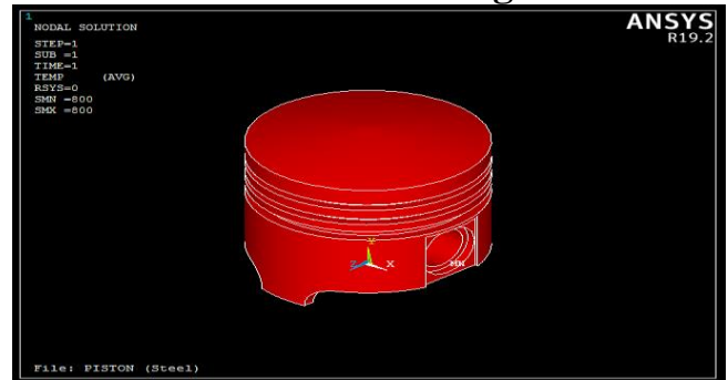
Fig. 7.11: Nodal Temperature of Piston – Forged Steel
